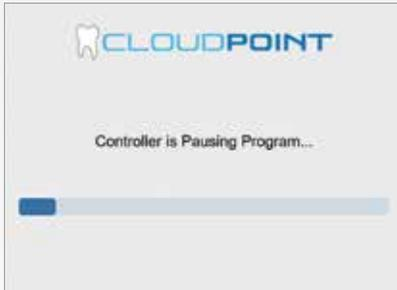
After pausing, press the RUN button to continue milling.
